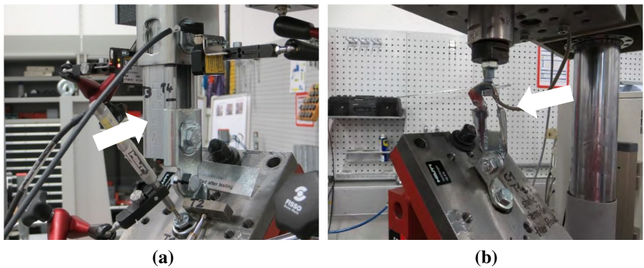
Fig. 15 Damage observed during tests on components C3 and C4: a X direction for component C3, b X direction for component C4
